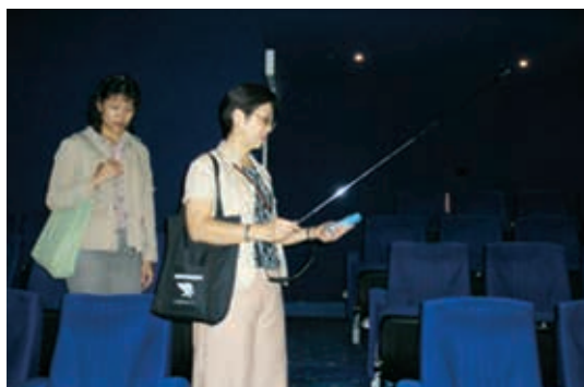
Managing hygiene in Places of Business – Testing air circulation speeds at movie theaters.
