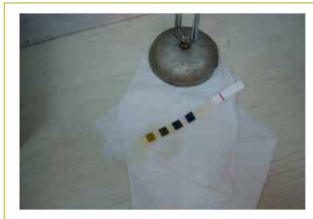
▲ 98年酸價試紙條測試炸油品質。 Testing of the acid value in oil used for deep fry with test paper.
